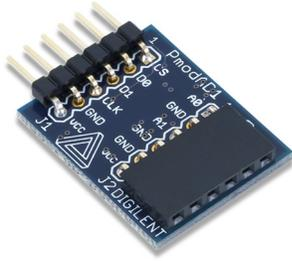
The Digilent Pmod AD1 (Revision G) is a two channel 12-bit analog-to-digital converter that features Analog Devices' AD7476A. With a sampling rate of up to 1 million samples per second, this Pmod™ is capable of excelling in even the most demanding audio applications.
