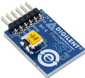
The Digilent Pmod MIC3 (Revision A) is small microphone module with a digital interface. With a Knowles Acoustics SPA2410LR5H-B MEMS microphone and Texas Instrument's ADCS7476 12-bit Analog-to-Digital Converter, you can capture your audio inputs with ease.
